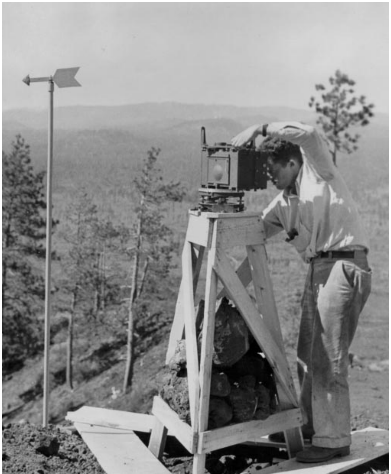
PHOTO-RECORDING transit set up for operation, without use of tripod legs. Ground setups like this could be made only on unimproved points being considered for use as a possible site for lookout location. Most camera setups were made with tripod on catwalks of stilt-mounted lookout stations. For ground stations camera could be set up on rooftop. For tall-tower stations rooftop setups were considered too dangerous. Most precise part of camera operation was leveling the instrument on the graduated azimuth ring, as operator is doing in photo. Camera was then oriented by sighting alidade on camera top to azimuth-identified topography on horizon.
